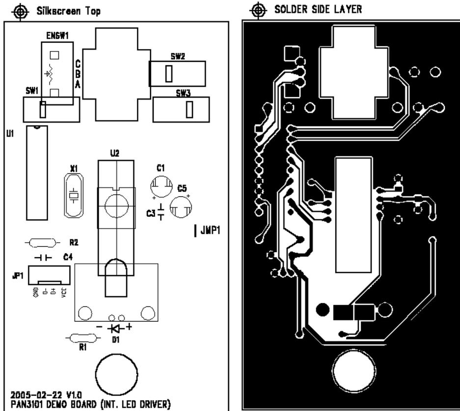
Figure 14. Example printed circuit board layout
