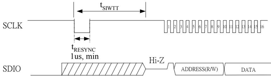
Figure 9. Re-synchronous serial interface using watchdog timer timeout
