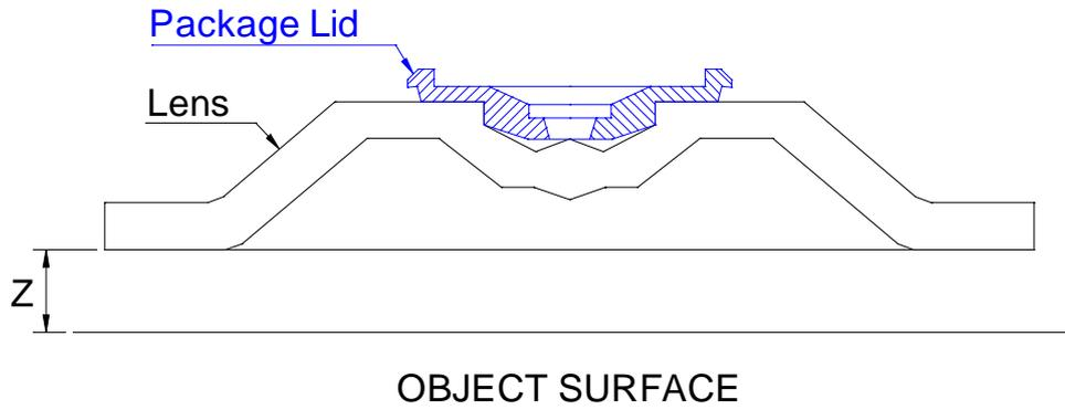
Figure 4. Distance from Lens Reference Plane to Surface
