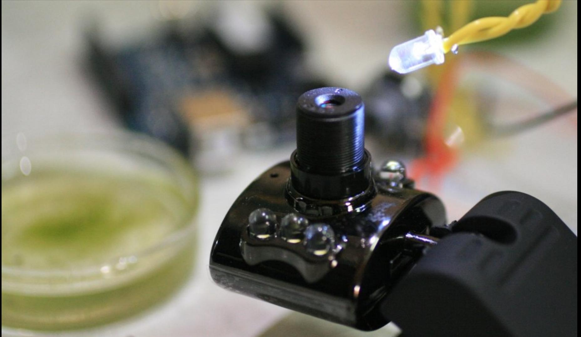
Repositioning of the lens turns a cheap webcam into a microscope
