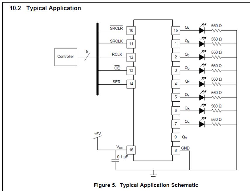
Figure 15 - Recommended LED Schematic from SN74HC595 Datasheet. Note current limiting 560  $\Omega$  resistors on output lines.
